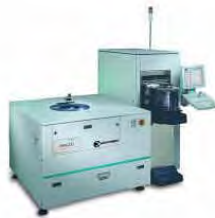
Wafer Probe
