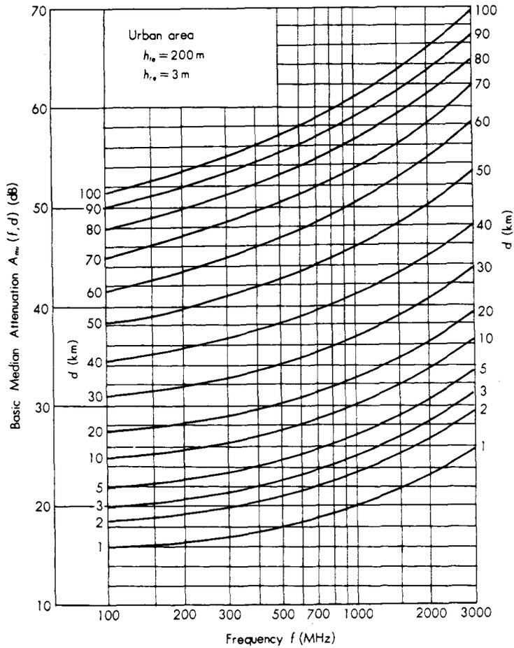
Figure 1. Prediction curve for basic median attenuation relative to free space in urban area over quasi-smooth terrain, referred to  $h_{te} = 200 \text{ m}$ ,  $h_{re} = 3 \text{ m}$ . From Okumura et al. (1968).
