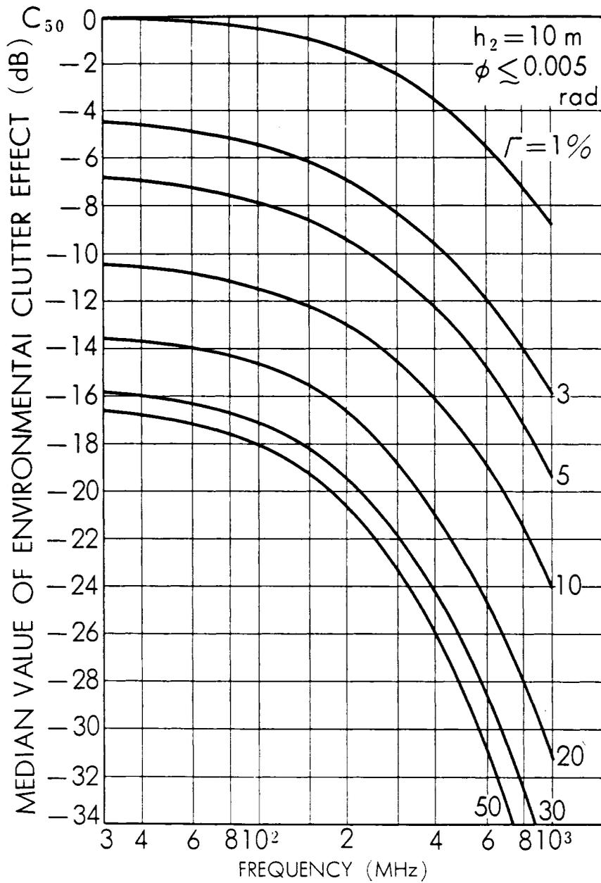
Figure 3. Median value of clutter effect as a function of frequency. From Kinase (1969).
