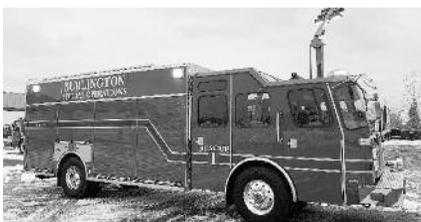
technical rescue trailer. The new Rescue One houses SCBA, a mobile cascade system, spare SCBA Cylinders, confined space rescue equipment, trench rescue equipment, swiftwater rescue equipment, and structural collapse equipment.
