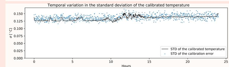
The temporal variation is a result of the fluctuating laser strength. An increase in the number of measurements and the Monte Carlo sample size result in a smaller spread of the standard deviation of the error (not shown here).
