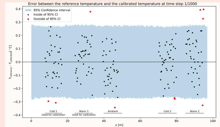
The 95% confidence interval becomes narrower if the acquisition time is increased.
