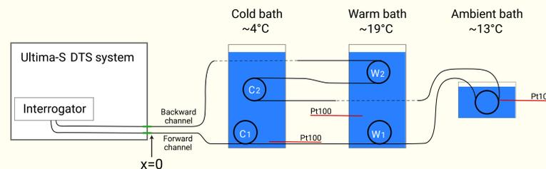
The temperature of the three baths is measured with external temperature sensors. The Stokes power and anti-Stokes power were measured 1000 times in one day with an acquisition time of 2 seconds. Measurements were made in the forward and backward direction to perform a double-ended calibration.
